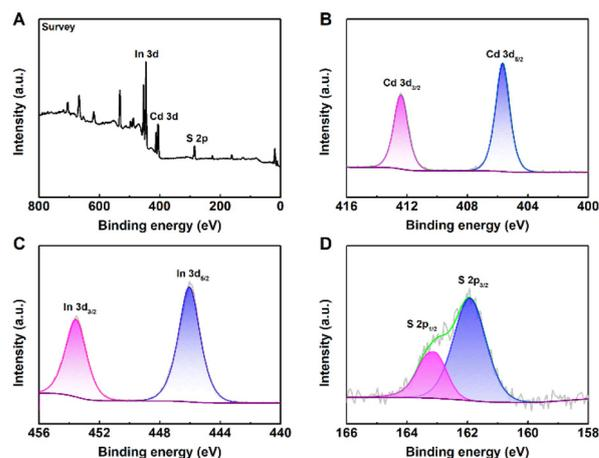
Fig. 2 XPS spectra of CdIn<sub>2</sub>S<sub>4</sub>@In<sub>2</sub>S<sub>3</sub> HMTs: (A) survey, (B) Cd 3d, (C) In 3d, and (D) S 2p.
