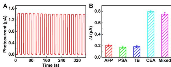
**Fig. 6** (A) Time-based photocurrent response of the proposed sensor under continuous “off–on–off” irradiation. (B) Selectivity of the designed sensor for the CEA target in comparison to other interfering substances at  $100 \text{ ng mL}^{-1}$ : AFP, PSA, TB, CEA, and the mixture containing AFP, PSA, TB and CEA.
