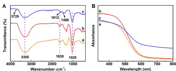
**Fig. 3** (A) FT-IR and (B) UV-vis diffuse reflectance spectra of  $\text{In}_2\text{S}_3$  HMTs (a),  $\text{CdIn}_2\text{S}_4@/\text{In}_2\text{S}_3$  HMTs (b), and MIP-capped  $\text{CdIn}_2\text{S}_4@/\text{In}_2\text{S}_3$  HMTs (c).
