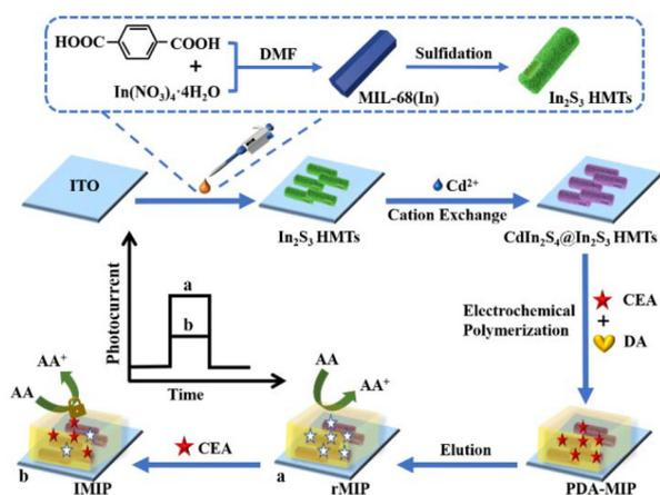
**Scheme 1** Schematic of the preparation procedures for the CdIn<sub>2</sub>S<sub>4</sub>@In<sub>2</sub>S<sub>3</sub> HMTs-based MIP-PEC sensor for CEA detection.
