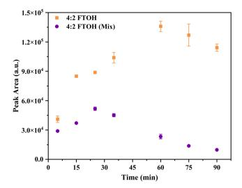
Fig. 2 Extraction time profiles of 4:2 FTOH extracted as part of a PFAS aqueous mixture (circle) and as an individual component (square). Extraction was conducted using an SPME-fiber in HS using an orbital shaker (OS); a temperature of 50 °C and 250 rpm was used for both incubation (25 min) and extraction, followed by a 5 min desorption. Analyte concentration was 2  $\mu$ g L<sup>-1</sup>.
