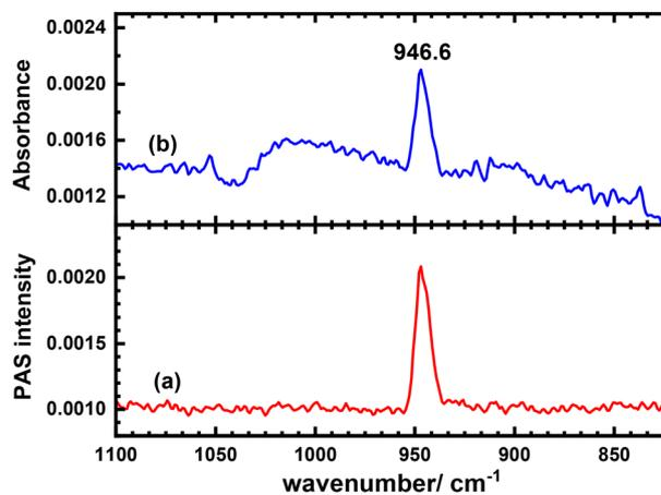
Fig. 5 IR spectra of 30 ppm  $\text{SF}_6/\text{N}_2$  recorded with a resolution of  $1\text{ cm}^{-1}$  near 298 K. (a) The PAS spectrum for a volume of 1 mL at 760 Torr. (b) The absorption spectrum for a volume of 1 mL injected into the gas cell (10 cm path length) filled with Ar at 760 Torr.
