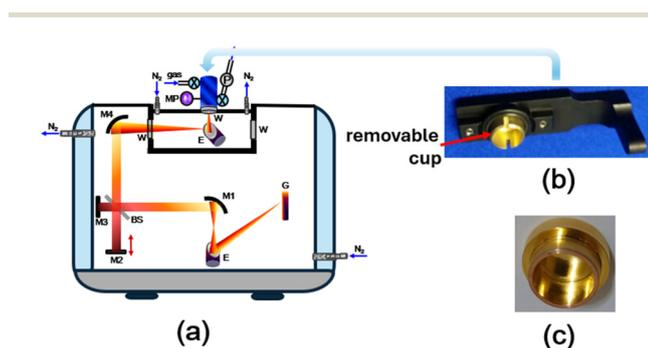
**Fig. 8** (a) Schematic diagram for the measurement of gaseous IR spectra with a photoacoustic apparatus. BS: KBr beam splitter; E: ellipsoid; G: globar; M1, M4 and M5: off-axis paraboloid mirrors; M2: scan mirror; M3: flat mirror; MP: microphone; P: pressure meter; W: KBr window. (b) Photograph of the removable brass cup of the gas cell. (c) Photograph of the in-house-fabricated cup from copper with a gold-plated surface.
