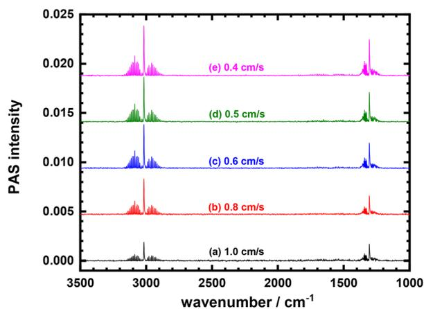
**Fig. 1** IR-PAS spectra of 5000 ppm CH<sub>4</sub>/air with a volume of 1 mL at 760 Torr near 298 K recorded with a resolution 2 cm<sup>–1</sup> for various FTIR scanning speeds of (a) 1.0, (b) 0.8 (Y-axis offset 0.0047), (c) 0.6 (Y-axis offset 0.0094), (d) 0.5 (Y-axis offset 0.0141) and (e) 0.4 cm s<sup>–1</sup> (Y-axis offset 0.0188).
