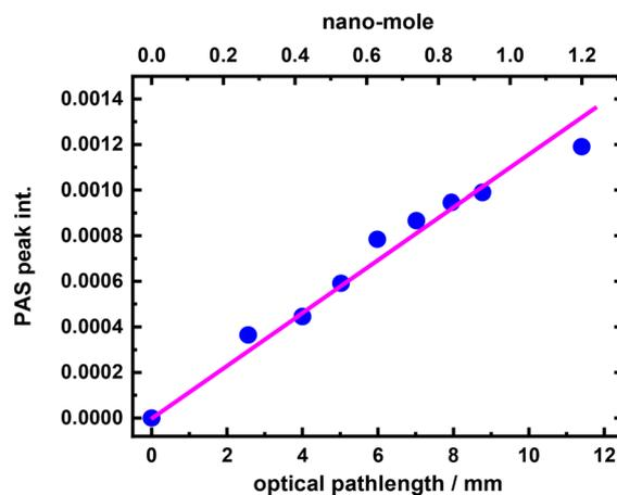
Fig. 7 Relationship of the intensity of the PAS peak centered at 946.6 cm<sup>-1</sup> vs. the optical path length (the lower axis in mm) of the gas cell and absolute quantity (the upper axis in nmol) of SF<sub>6</sub> recorded with a resolution of 2 cm<sup>-1</sup> from the sample of 30 ppm SF<sub>6</sub>/N<sub>2</sub> under 760 Torr near 298 K.
