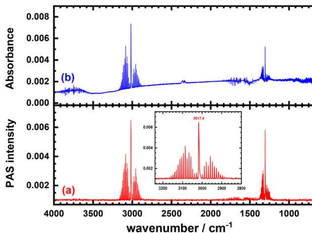
Fig. 3 IR spectra of 5000 ppm  $\text{CH}_4/\text{air}$  recorded with a resolution  $1\text{ cm}^{-1}$ . (a) The PAS spectrum for a volume of 1 mL at 760 Torr near 298 K. (b) The direct absorption spectrum for a volume of 1 mL injected into a gaseous Ar cell (10 cm in path length) at 760 Torr near 298 K.
