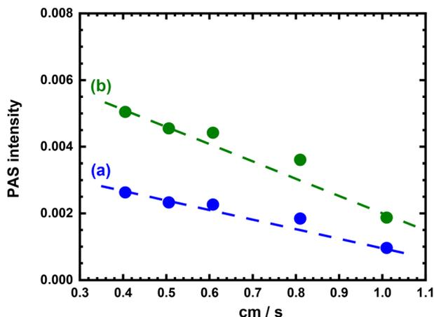
Fig. 2 Relationships of intensities of IR-PAS spectra for peaks at  $3017\text{ cm}^{-1}$  vs. scanning speed of the moving mirror in the FTIR system for 5000 ppm  $\text{CH}_4/\text{air}$  recorded with resolutions of (a)  $8\text{ cm}^{-1}$  and (b)  $2\text{ cm}^{-1}$ .
