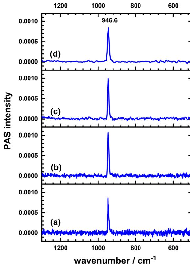
Fig. 4 IR-PAS spectra of 30 ppm  $\text{SF}_6/\text{N}_2$  for a volume of 1 mL at 760 Torr near 298 K in the wavenumber region  $1300\text{--}500\text{ cm}^{-1}$  measured with resolutions of (a) 1, (b) 2, (c) 4, and (d)  $8\text{ cm}^{-1}$ .
