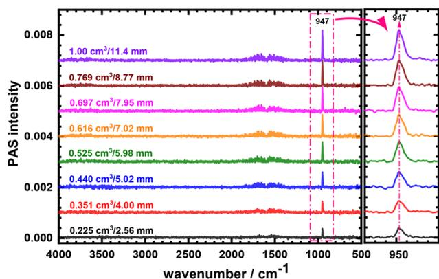
Fig. 6 IR-PAS spectra of 30 ppm SF<sub>6</sub>/N<sub>2</sub> measured at various volumes/optical path lengths (Y-axis offsets 0.001, respectively) with a resolution of 2 cm<sup>-1</sup> under 760 Torr near 298 K.
