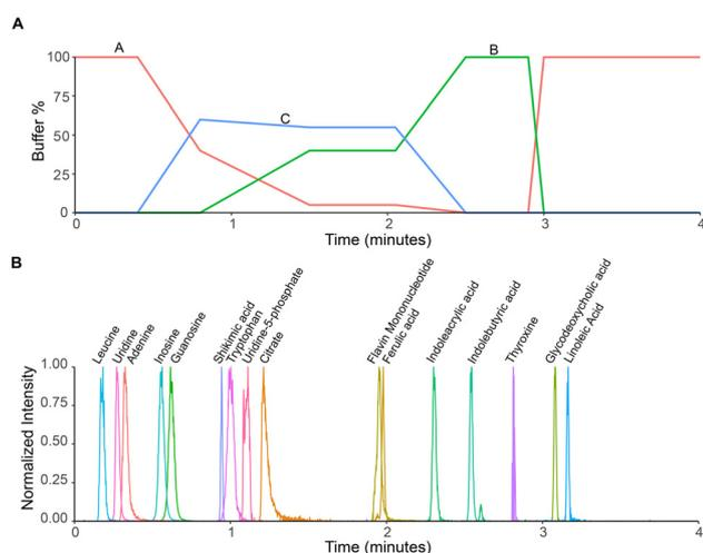
**Fig. 1** Representation of mixed-mode chromatographic gradient. (A) Gradient profile with the relative concentrations of solvent A (red): 5  $\mu$ M medronic acid in water, solvent B (green): 0.1% v/v formic acid in methanol; and solvent C (blue): 5 mM ammonium formate and 0.1% v/v formic acid in water. (B) Examples of chromatographic peak shapes.
