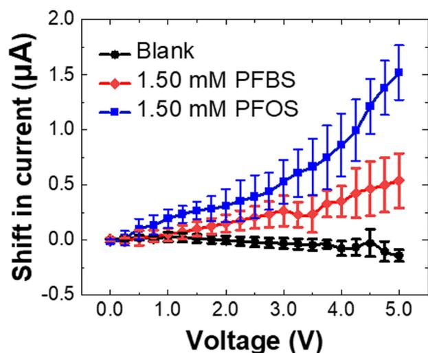
Fig. 3 Plot showing the CVC shift for blank (10 mM Tris-HClO<sub>4</sub>, black) PFBS (4 carbons, red), and PFOS (8 carbons, blue) in 10 mM Tris-HClO<sub>4</sub> (pH 8.35) ( $n \geq 3$ ).
