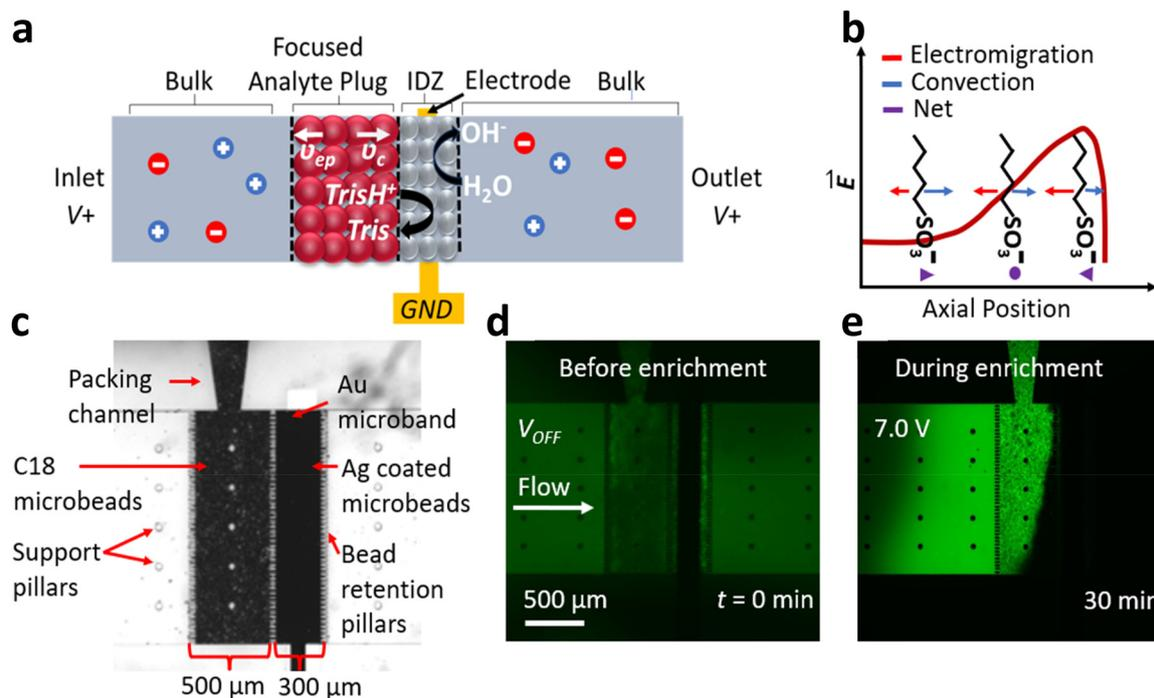
**Fig. 4** (a) Schematic showing the mechanism of fICP. (b) Demonstration of the focusing of PFOS within an electric field gradient, especially at the interface of the IDZ in the presence of convection. (c) Brightfield micrograph of C18 and Ag bead beds located at the center of the microchannel. (d and e) Fluorescence micrographs of the enrichment of 100  $\mu\text{M}$  fluorescein dye in 10 mM Tris-HClO<sub>4</sub> under an applied voltage of  $V^+ = 7.0$  V at  $t = 0$  and 30 min.
