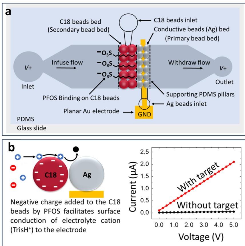
**Scheme 1** (a) Illustration of overall device design (top view), (b) the suggested mechanism for enhanced system conductance due to PFOS adsorption on the C18 beads. An increase in the negative charge present on the C18 beads promotes surface conduction of cations to the conductive silver beads, resulting in a shift in current.
