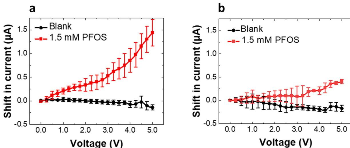
**Fig. 1** Plots demonstrating the shift in current as a function of voltage for the adsorption of 1.5 mM PFOS on C18 beads in 10 mM Tris-HClO<sub>4</sub> (pH 8.35) (a) after 30 min of PFOS flowing (0 mM black trace, 1.5 mM red trace,  $n \geq 3$ ) and (b) after 10 min of rinsing (after PFOS flowing) with background electrolyte solution (0 mM black trace, 1.5 mM red trace,  $n \geq 3$ ).
