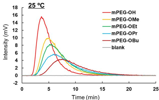
Fig. 3 Chromatograms of single-end type analytes at 25 °C.
