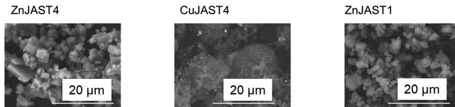
Fig. 1 SEM images of the prepared MOF crystals.
