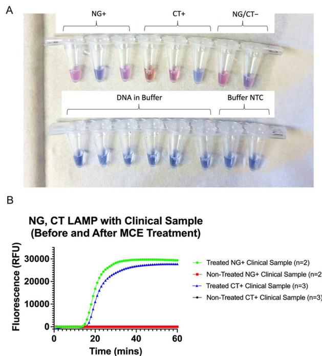
**Fig. 3** Filtration of clinical vaginal samples enabled in-tube LAMP reactions. (A) Comparison of lyophilized LAMP reagents rehydrated with clinical vaginal samples (top row) and buffer samples (bottom row). (B) Quantified averaged *Neisseria gonorrhoeae* (NG) ( $n = 2$ ) and *Chlamydia trachomatis* (CT) ( $n = 3$ ) signals. LAMP results for the QMA membrane comparing treated and non-treated clinical vaginal samples (see Fig. S5 for all reaction curves).
