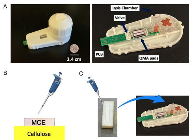
**Fig. 1** A UbiNAAT integrated device. (A) Fully assembled device (left) and device without top enclosure (right). (B) A mixed cellulose ester (MCE) filtration setup with a cellulose wicking membrane. (C) Transfer of the MCE membrane post-filtration and rinsing into the lysis chamber of the UbiNAAT device. Images in (B) and (C) are not to scale.
