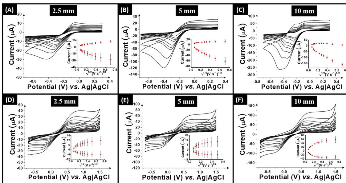
Fig. 5 Cyclic voltammogram scan rate study (5–500  $\text{mV s}^{-1}$ ) with  $[\text{Ru}(\text{NH}_3)_6]^{3+}$  (1 mM in 0.1 M KCl) performed in the 40 wt% CB/TPU filaments with different sizes. Inset: the Randles-Ševčík plot: (A) 2.5 mm; (B) 5 mm; (C) 10 mm. Scan rate study (5–500  $\text{mV s}^{-1}$ ) with  $[\text{Fe}(\text{CN})_6]^{4-/3-}$  (1 mM in 0.1 M KCl) performed in the 40 wt% CB/TPU filaments with different sizes. Inset: the Randles-Ševčík plot: (D) 2.5 mm; (E) 5 mm; (F) 10 mm.
