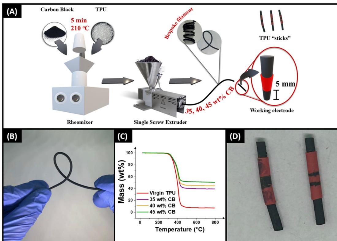
**Fig. 1** (A) Schematic representation of filament production. (B) Photograph highlighting the low temperature flexibility of the 45 wt% CB/TPU filament. (C) Thermogravimetric analysis (TGA) of the virgin TPU and the 35, 40 and 45 wt% CB filaments. (D) Photographs of electrodes in the "stick" designs.
