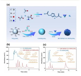
Fig. 3 (a) A synthetic scheme for the preparation of [BCMIM]Cl-Zr-MOF@SiO2. Chromatograms of (b) PAHs and (c) sulfonamides on the [BCMIM]Cl-Zr-MOF@SiO<sub>2</sub> column and the Zr-MOF@SiO<sub>2</sub> column. Reproduced with permission from ref. 86. Copyright 2025, Elsevier.
