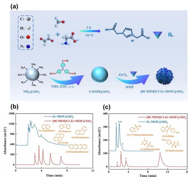
**Fig. 3** (a) A synthetic scheme for the preparation of [BCMIM]Cl-Zr-MOF@SiO<sub>2</sub>. Chromatograms of (b) PAHs and (c) sulfonamides on the [BCMIM]Cl-Zr-MOF@SiO<sub>2</sub> column and the Zr-MOF@SiO<sub>2</sub> column. Reproduced with permission from ref. 86. Copyright 2025, Elsevier.
