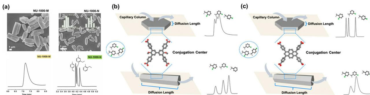
**Fig. 4** (a) SEM and gas chromatograms of NU-1000-M and NU-1000-N. Reproduced with permission from ref. 89. Copyright 2022, American Chemical Society. Separation performance of (b) PCN-MOFs and (c) NU-MOFs influenced by both diffusion length and interaction centers. Reproduced with permission from ref. 91. Copyright 2022, John Wiley and Sons.
