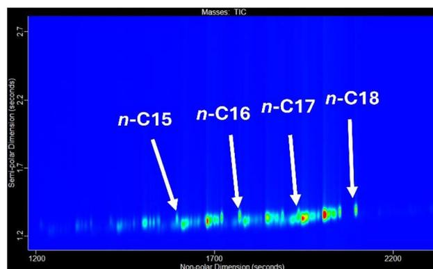
Fig. 2 Two-dimensional total ion current chromatogram (TICC) contour plot of the GCxGC-MS analysis of diluted HVO 1.
