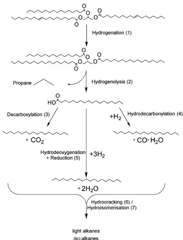
Fig. 1 Simplified reaction scheme for the production of HVOs from triacylglycerides.
