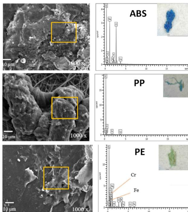
Fig. 6 SEM images and corresponding EDX spectra of ABS, PP, and PE.<sup>34</sup>
