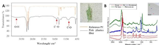
Fig. 7 (A) FTIR spectra recorded from reference PE and pink plastics fiber.<sup>34</sup> (B) Raman spectra of reference PE, fish bone standard and MPs sample.<sup>35</sup>
