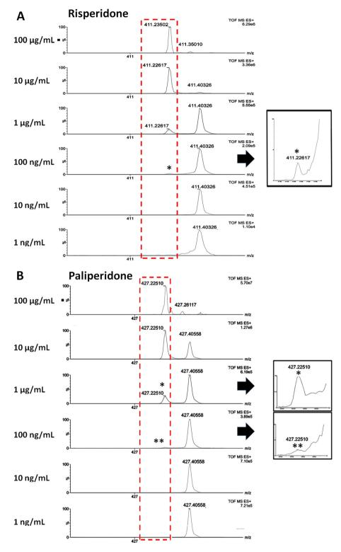
Fig. 3 SICRIT ionisation of serial dilutions of risperidone (A) and paliperidone (B) spotted in fingermarks. Both risperidone and paliperidone were detectable down to 100 ng mL<sup>-1</sup>. The inset \* in both panels A and B show a viable risperidone and paliperidone ion signal, respectively.
