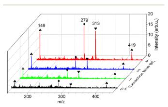
Fig. 4 Mass spectra of acetonitrile extract obtained from a disposable plastic tip dropper in the laboratory. A Protonated phthalic anhydride ions (m/z = 149),  $\spadesuit$  DBP (m/z = 279),  $\heartsuit$  BBP (m/z = 313), and  $\spadesuit$  DINP (m/z = 313)z = 419)
