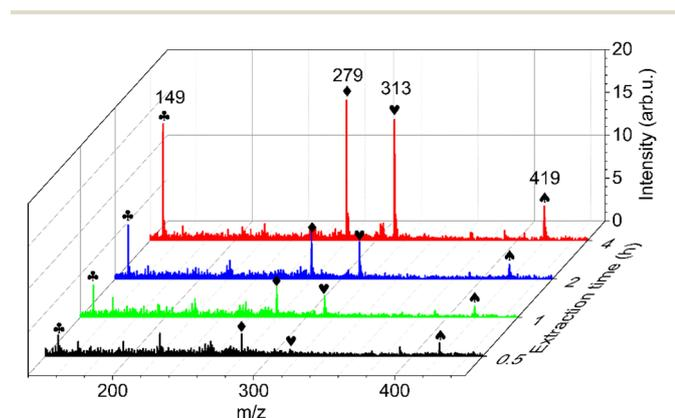
Fig. 4 Mass spectra of acetonitrile extract obtained from a disposable plastic tip dropper in the laboratory. ♣ Protonated phthalic anhydride ions ( $m/z = 149$ ), ♠ DBP ( $m/z = 279$ ), ♥ BBP ( $m/z = 313$ ), and ♦ DINP ( $m/z = 419$ ).
