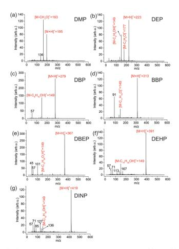
Fig. 3 Mass spectra of plasticizers in positive ion mode. (a) DMP, (b) DEP. (c) DBP. (d) BBP. (e) DBEP. (f) DEHP. and (g) DINP. The above data are from standard solutions in ACN/H<sub>2</sub>O (50/50, v/v) at a concentration of 100 ppm.
