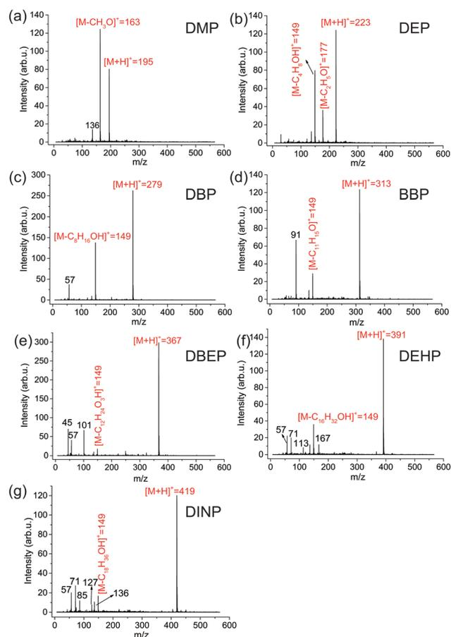
Fig. 3 Mass spectra of plasticizers in positive ion mode. (a) DMP, (b) DEP, (c) DBP, (d) BBP, (e) DBEP, (f) DEHP, and (g) DINP. The above data are from standard solutions in ACN/ $H_2O$  (50/50, v/v) at a concentration of 100 ppm.
