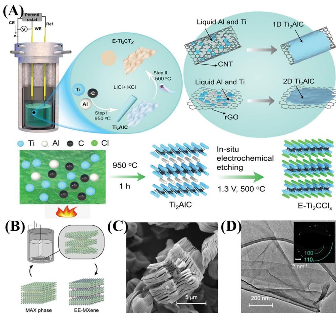
**Fig. 4** (A) Schematic illustration of the fabrication process of  $Ti_2AlC$  and  $E-Ti_2CT_x$ . Reproduced from ref. 37 with permission from WILEY, copyright 2023. (B) Schematic illustration of the setup to etch  $EE-Ti_3C_2$ . (C) SEM image of  $EE-Ti_3C_2$  multilayer powder. (D) TEM image of a delaminated  $EE-Ti_3C_2$  flake. Reproduced from ref. 38 with permission from the Royal Society of Chemistry, copyright 2024.
