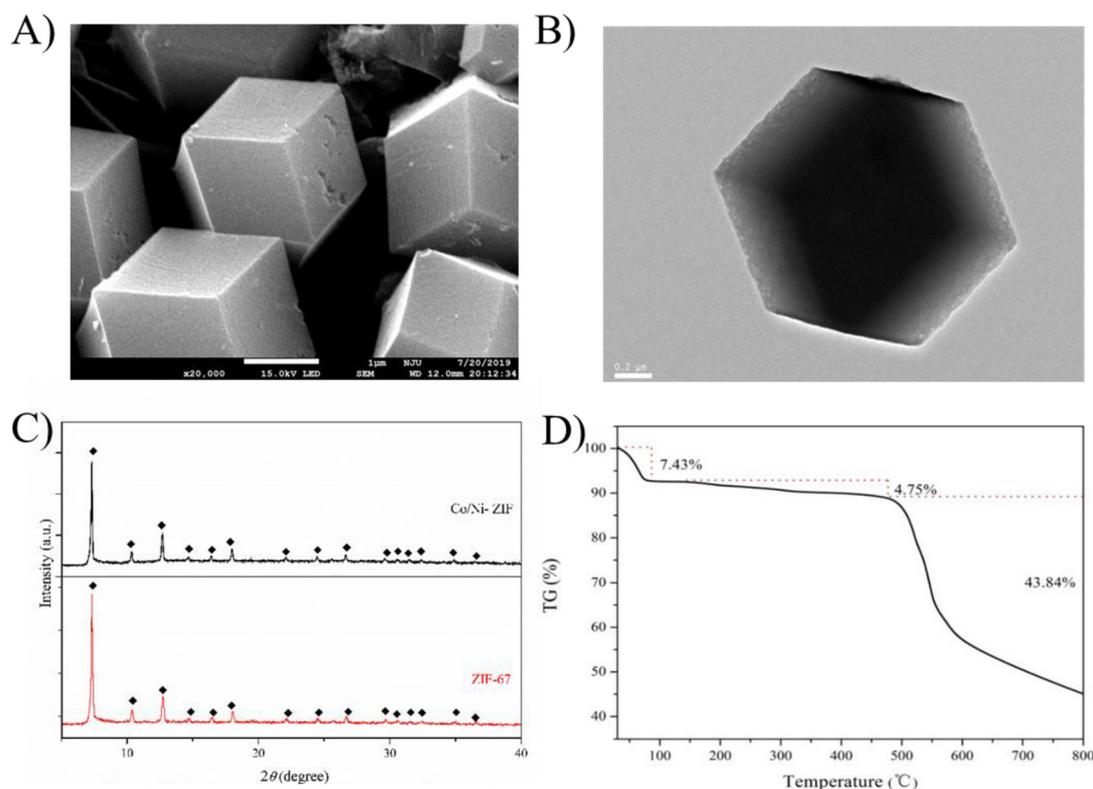
**Fig. 1** SEM (A) and TEM (B) images of Co/Ni-ZIF; XRD patterns of ZIF-67 and Co/Ni-ZIF (C); and TGA curve of Co/Ni-ZIF (D). ZIF-67: Co(NO<sub>3</sub>)<sub>2</sub>: Ni(NO<sub>3</sub>)<sub>2</sub>, 5:0; Co/Ni-ZIF: Co(NO<sub>3</sub>)<sub>2</sub>: Ni(NO<sub>3</sub>)<sub>2</sub>, 1:1.
