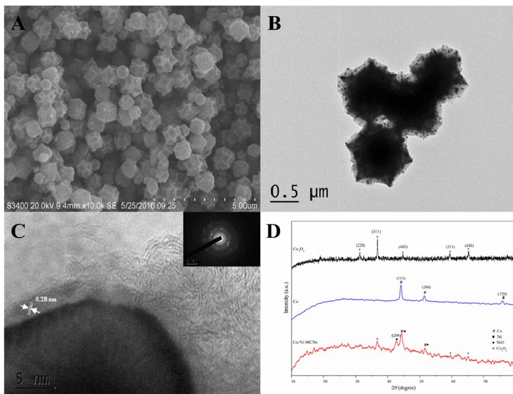
Fig. 2 SEM (A), TEM (B) and HR-TEM images (C) of Co/Ni-MCNs; XRD patterns of Co/Ni-MCNs, as well as Co and Co<sub>3</sub>O<sub>4</sub> nanopowders (D).
