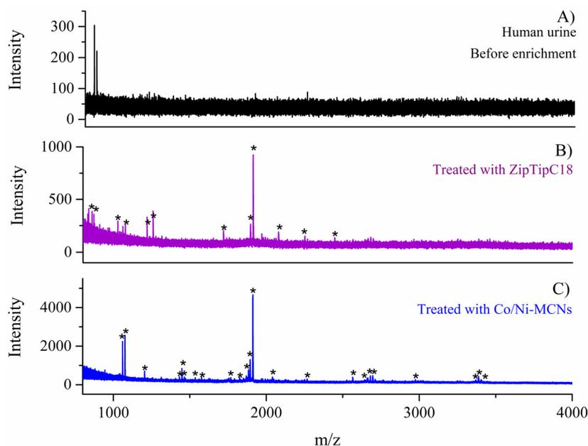
Fig. 5 MS spectra of human urine before enrichment (A) and after enrichment with ZipTipC18 (B) and Co/Ni-MCNs (C).
