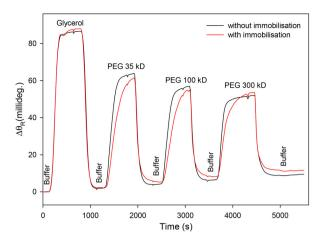
Fig. 9 Shifts in resonance angle  $(\Delta\theta_{R})$  of LWs comprising waveguide films without and with immobilised half antibody fragments in response to solutions of PEGs of different molecular weights.
