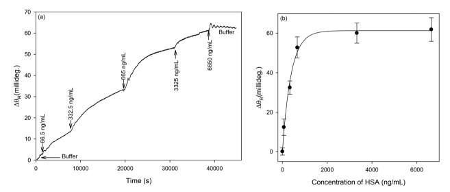
Fig. 10 (a) Real-time measurement of shift in resonance angle ( $\Delta\theta_{\rm R}$ ) (sensor-reference) of the LW with increase in concentration of HSA from 66.5 ng ml<sup>-1</sup> (or 1 nM) to 6650 ng ml<sup>-1</sup> (or 100 nM) and (b) shift in resonance angle versus concentration of HSA where the error bars for each concentration of the protein were calculated using 3 replicates on a LW biosensor and error bars on blank were calculated using 11 LWs.
