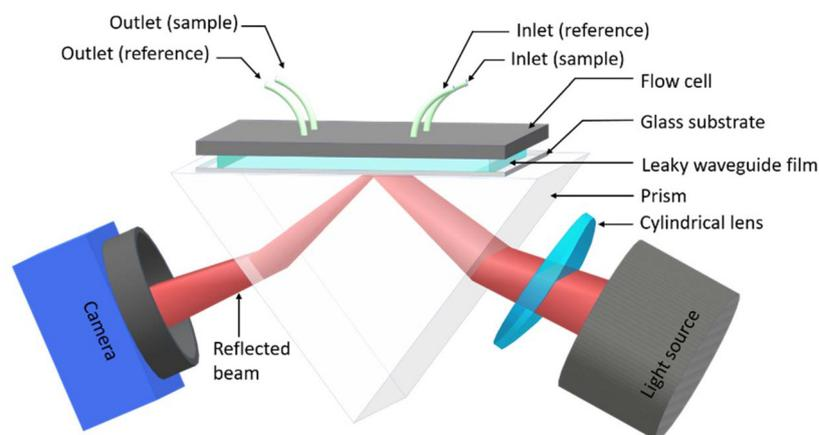
Fig. 1 Schematic of the leaky waveguide instrumentation.
