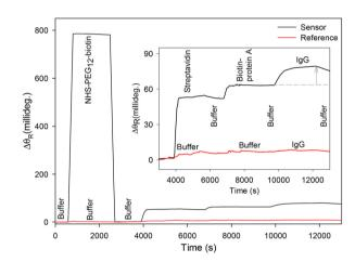
Fig. 6 Shifts in resonance angle  $(\Delta\theta_{\rm R})$  as different solutions used in immobilisation strategy 1 were flowed in the sensor and reference flow channels of the flow cell on LW.
