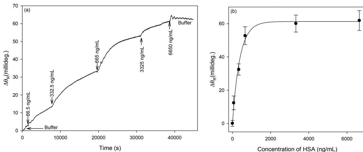
**Fig. 10** (a) Real-time measurement of shift in resonance angle ( $\Delta\theta_R$ ) (sensor–reference) of the LW with increase in concentration of HSA from  $66.5 \text{ ng mL}^{-1}$  (or  $1 \text{ nM}$ ) to  $6650 \text{ ng mL}^{-1}$  (or  $100 \text{ nM}$ ) and (b) shift in resonance angle versus concentration of HSA where the error bars for each concentration of the protein were calculated using 3 replicates on a LW biosensor and error bars on blank were calculated using 11 LWs.
