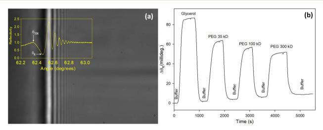
Fig. 2 (a) Two- and one-dimensional reflectivity curves and (b) shift in resonance angle  $(\Delta\theta_R)$  for 0.5% (v:v) glycerol and 0.5% (w:v) PEG solutions of an optimised LW.
