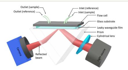
Fig. 1 Schematic of the leaky waveguide instrumentation.
