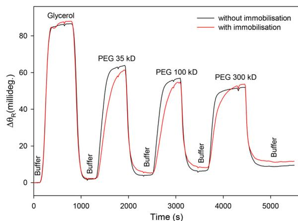
**Fig. 9** Shifts in resonance angle ( $\Delta\theta_R$ ) of LWs comprising waveguide films without and with immobilised half antibody fragments in response to solutions of PEGs of different molecular weights.
