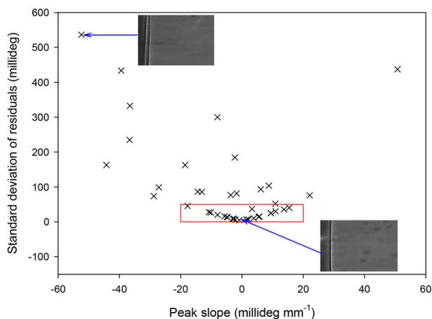
**Fig. 4** Plot of non-uniformity versus tilt in the position of resonance angle for hydrogels films of 42 LW devices fabricated using casting where scatter points in the red box are the devices that passed the quality check.
