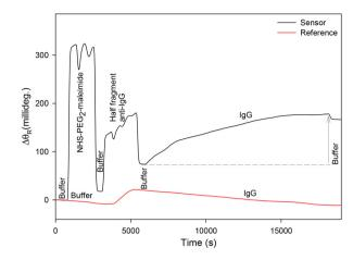
Fig. 8 Shifts in resonance angle  $(\Delta\theta_{\rm R})$  as different solutions used in immobilisation strategy 3 were flowed in the sensor and reference flow channels of the flow cell on LW.
