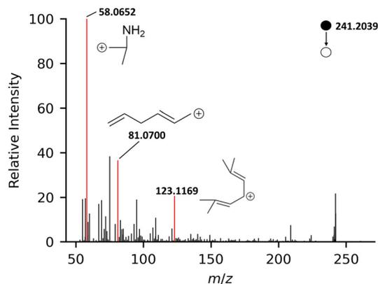
Fig. 3 High-resolution MS/MS  $[M + 2H]^{2+}$  spectrum of BTMPS, with the three selected confirming ions highlighted.
