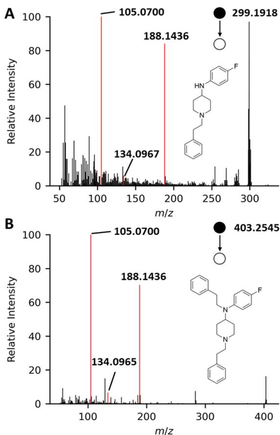
**Fig. 6** High-resolution PS-MS/MS  $[M + H]^+$  spectrum of (A) F-ANPP with the three selected confirming ions highlighted, and (B) fluoro-phenethyl-ANPP with three selected confirming ions highlighted.
