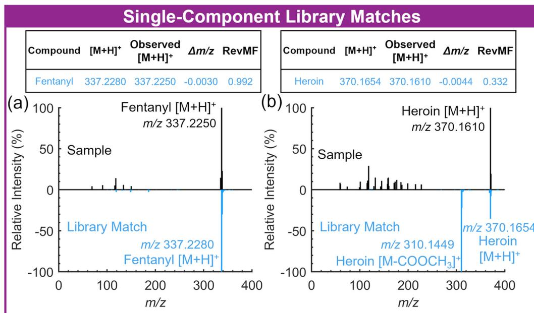
**Fig. 4** Single-spectrum matching (*i.e.*, low fragmentation) of (a) fentanyl [DBDI parameters: TD: 250 °C, DBDI voltage: 1400 V, DBDI frequency: 15 kHz, inlet pump: 25%] and (b) heroin [acetone-assisted VUV photoionization parameters: ion-molecule reactor temp: 50 °C, perm tube flow: 150 cm<sup>3</sup> min<sup>-1</sup>, VUV voltage: 1600 V, inlet pump: 5%] using the DIT with NIST DART-MS Forensics Database library. DIT search results and match factors displayed in insets.
