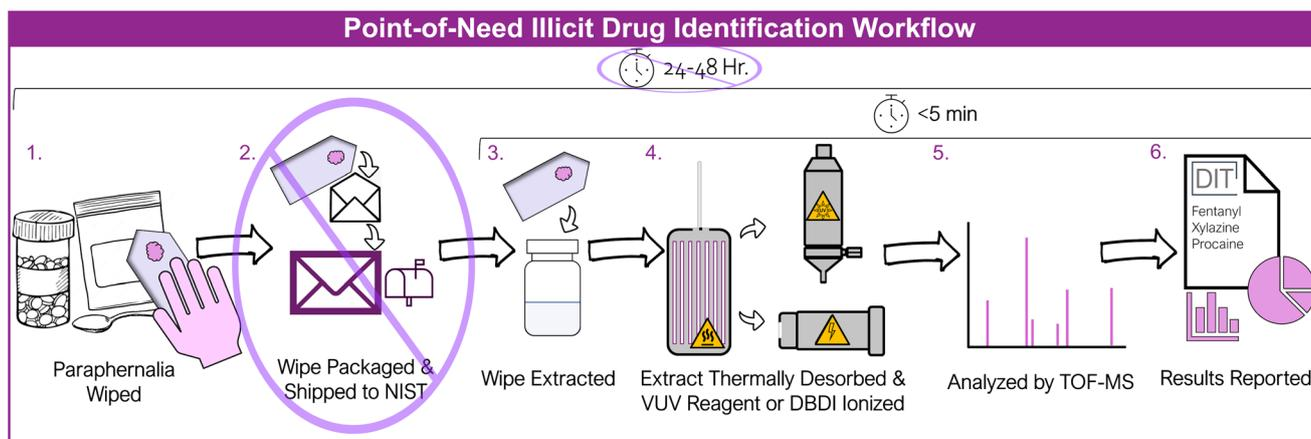
**Fig. 1** Schematic representation of the NIST RaDAR workflow and overall reduction in process time by on-site analysis. Step 1: swipe sample collection from paraphernalia, 2: packaging of sample-laden wipes and shipping to NIST, 3: solvent extraction of wipes, 4: thermal desorption and ionization of samples, 5: TOF-MS analysis, and 6: Library matching and preliminary identification.
