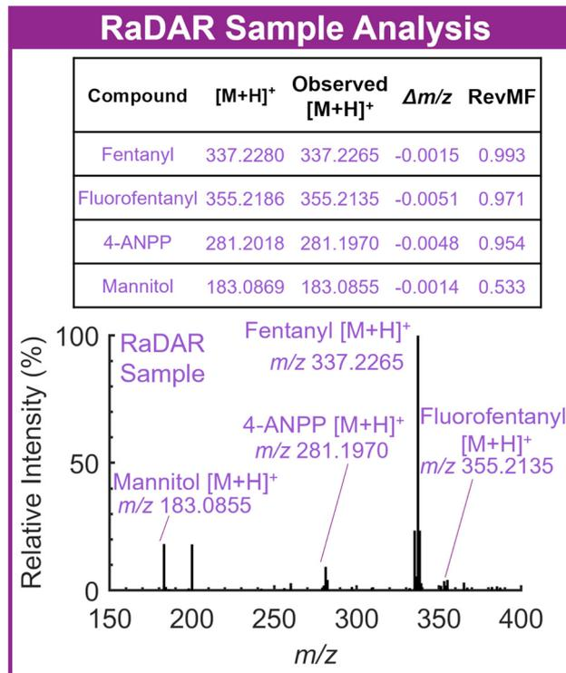
**Fig. 5** Low fragmentation DBDI-MS mass spectra of RaDAR sample #3 with matched compounds labeled. Insets display search results and match scores from the DIT. Parameters: TD: 250 °C, DBDI voltage: 1400 V, DBDI frequency: 15 kHz, inlet pump: 25%.
