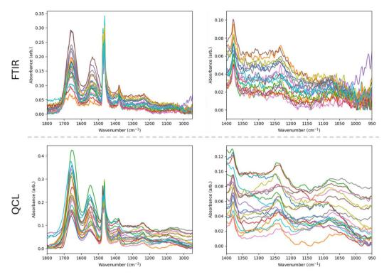
Fig. 2 Comparison of 20 randomly sampled raw (unprocessed) spectra collected on FTIR (top) and QCL (bottom) systems. Plots are generated for full fingerprint regions (1800-1000 cm<sup>-1</sup>) and lower wavenumber regions (1400-1000 cm<sup>-1</sup>).
