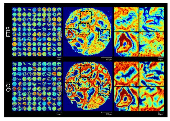
Fig. 1 Comparison of amide I peak integration (1600–1700 cm<sup>-1</sup>) images for 100 cores imaged on d FTIR and QCL instruments (left). A single core is highlighted (white dotted lines, left) in greater detail (centre), with four selections from within the core also plotted for comparison of image quality (right).
