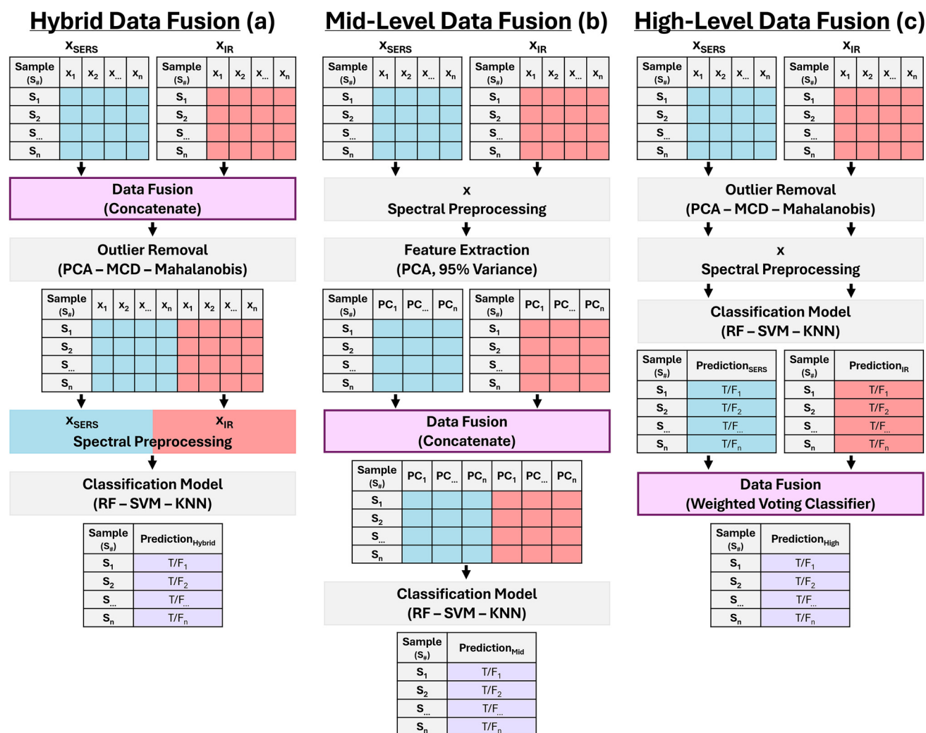
Fig. 2 Flowchart of data fusion strategies for (a) hybrid, (b) mid-level, and (c) high-level fusion approaches. The presentation style has been adapted from ref. 63.
