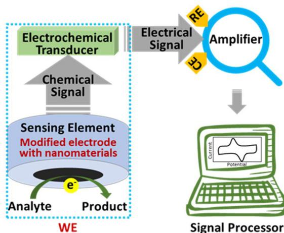
Fig. 2 Schematic diagram of a typical electrochemical sensor.
