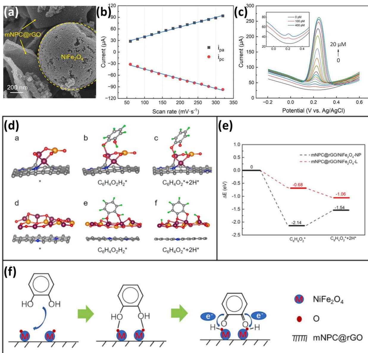
Fig. 7 (a) SEM image of mNPC@rGO/NiFe<sub>2</sub>O<sub>4</sub>. (b) The dependence of redox current on the scan rate. (c) DPVs of CGA quantitative analysis on mNPC@rGO/NiFe<sub>2</sub>O<sub>4</sub>/GCE. Reprinted by permission from ref. 34. Copyright, 2023, Elsevier.
