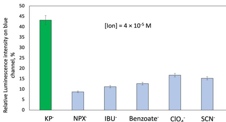
Fig. 7 Relative luminescence intensity of membrane Mb5 sensing spots on the blue channel in the presence of equal amounts of  $\text{KP}^-$ , naproxen ( $\text{NPX}^-$ ), ibuprofen ( $\text{IBU}^-$ ), benzoate ( $\text{Benzoate}^-$ ),  $\text{ClO}_4^-$  and  $\text{SCN}^-$  interfering anions.  $[\text{I}_{\text{on}}] = 4 \times 10^{-5}$  M, pH = 7.0, Tris 0.005 M, and  $\lambda_{\text{exc}} = 365$  nm.
