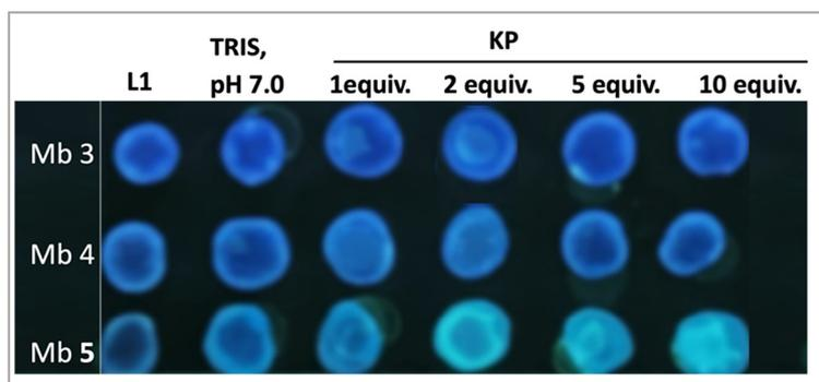
**Fig. 4** Photogram of L1-based all-solid-state optodes deposited on the glass support GS to increasing concentrations of KP (1–10 equiv.) on 0.005 M Tris pH 7.0 background solution. In membrane Mb3, the L1 ligand is in its not-protonated form, and in membranes Mb4 and Mb5, 1.5 and 2.8 equiv. of TFA, respectively, were added to protonate L1 directly in the membrane phase. The image was acquired from 10 cm distance with a common smartphone,  $\lambda_{\text{exc}} = 365$  nm.
