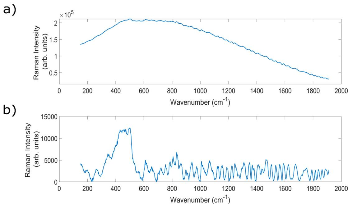
**Fig. 1** (a) An example of a highly fluorescent, raw Raman spectrum of porcine liver (a particularly fluorescent organ) taken using a fibre optic Raman probe at 830 nm. Mean of  $15 \times 40$  second spectral measurements. (b) Corresponding baselined spectrum.
