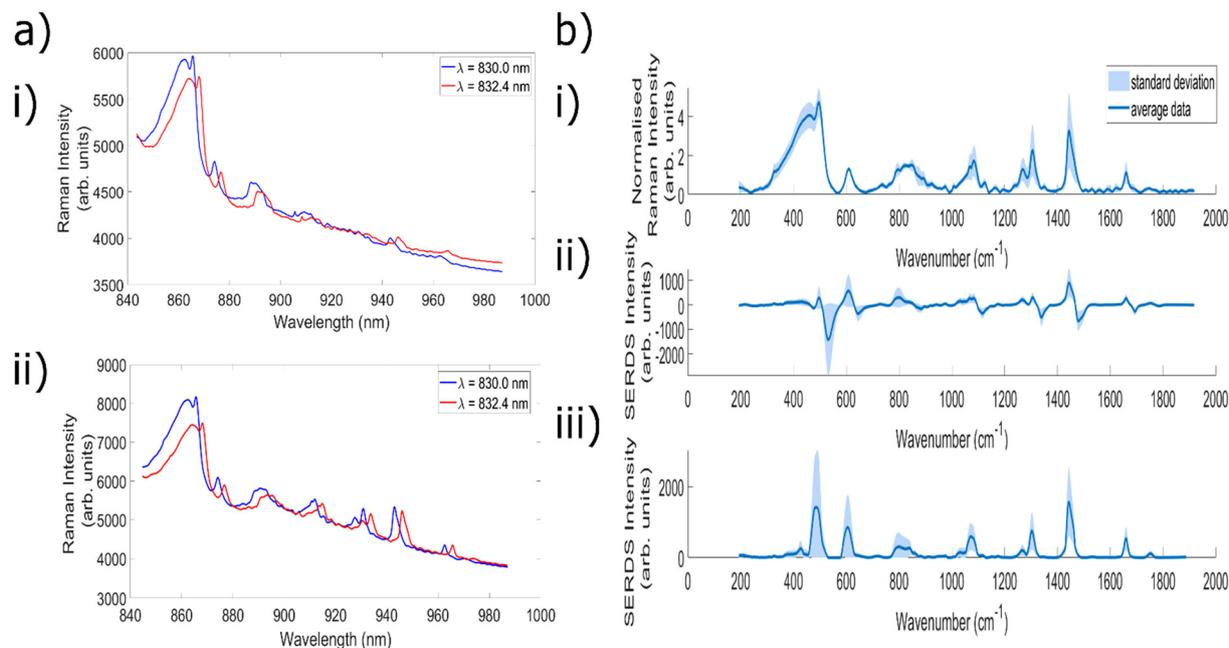
**Fig. 6** (a) Average: (i) cancerous, (ii) reactive lymph node spectra, taken with 830.0 nm and 832.4 nm excitation using needle probe #2. Acquisition time =  $5 \times 10$  s. (b) average: (i) standard Raman, (ii) SERDS difference and (iii) SERDS reconstructed spectra from the reactive lymph node measured. Acquisition time standard Raman spectra =  $5 \times 20$  s. Acquisition time SERDS spectra =  $5 \times 20$  s.
