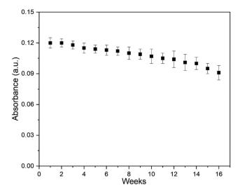
Fig. 6 Absorbance of oxidized TMB solutions at 652 nm for 16 weeks. For every data point, a fresh solution of TMB was prepared and reacted in the presence of Cu nanozymes and 10  $\mu M$  H<sub>2</sub>O<sub>2</sub> for 30 minutes. The nanocubes were stored in water after each use to avoid oxidation. Error bars represent the standard deviation of three replicate measurements.
