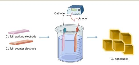
Fig. 1 Electrochemical synthesis of Cu nanocubes at 8V in 1 M CuCl<sub>2</sub> electrolyte.
