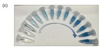
Fig. 4 Detection of  $H_2O_2$  and sarcosine. (a) Linear calibration curves for varying concentrations of  $H_2O_2$  with TMB at 1 mM, and (b) varying concentrations of sarcosine using sarcosine oxidase and Cu nanozymes with TMB at 1 mM. Error bars are standard deviations from three replicate measurements. (c) Corresponding images of visible color in the presence of varying concentrations of sarcosine.
