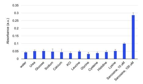
Fig. 5 Selectivity of the Cu nanozyme sensing platform. The concentration of all compounds was 100 μM except for the one experiment with sarcosine at 10 µM as indicated in the graph. All error bars were estimated from three replicate measurements.
