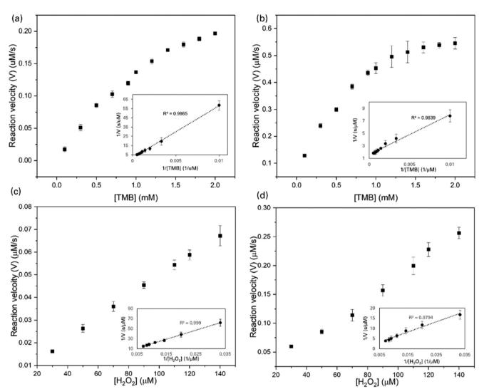
Fig. 3 Characterization of reaction kinetics. Initial reaction velocity is plotted as a function of TMB (a and b) and  $H_2O_2$  (c and d) substrate concentration for pristine Cu foil (a and c) and etched Cu foil (b and d), with inset Lineweaver–Burk plots showing good fitting to the Michaelis–Menten equation. Standard deviations are from three replicate measurements.
