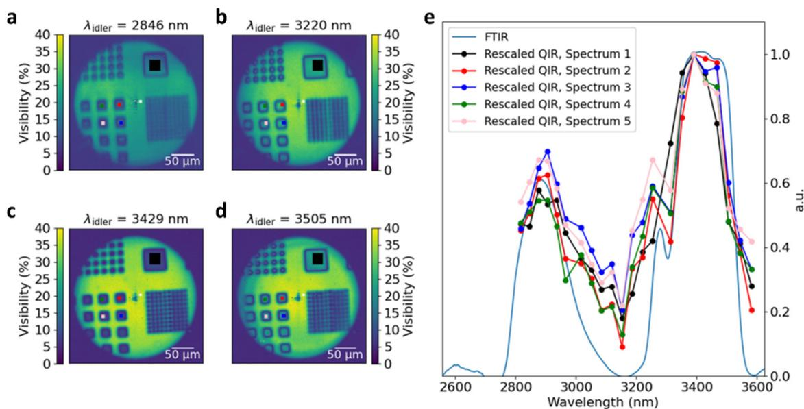
**Fig. 4** (a–d) IR images of the microfluidic chip without being filled with water, taken using a Q-IR microscopy system. The images in (a–d) show the visibility map of the interference pattern at probe (idler) wavelengths of 2846 nm, 3220 nm, 3429 nm, and 3505 nm, respectively. (e) IR absorption spectra of the SU-8 photoresist calculated for five square regions of interest highlighted by different colours in (a)–(d): black, green, red, pink, and blue.
