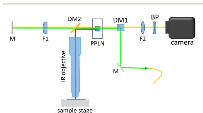
**Fig. 3** Scheme of the Q-IR imaging set-up (Michelson interferometer): M is a mirror, DM1 and 2 are dichroic mirrors, F1 and 2 are lenses, and BP is a bandpass filter.
