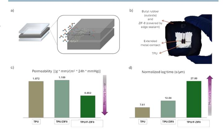
Fig.2 Schematich illustration of the tortuous pathways mechanism that hinders transverse water molecule permeation (a); encapsulated device (b) permeability (c) and lag time (d) of reference samples, ZIF8, and modified F-ZIF8 measured at room temperature (RT) and 85% relative humidity (RH).
