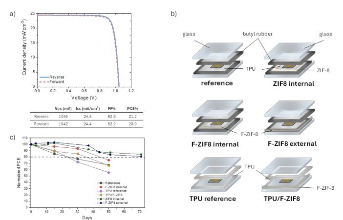
Fig.3 J-V curve of reference sample after the encapsulation (a); schematic representation of the different layouts used (b); normalized efficiency of encapsulated PSCs over time under aging test conducted at 95%RH and RT (c).
