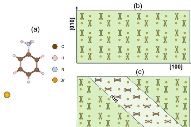
Fig. 1 crystal structure of  $P2_1/c$  AniHBr. (a) Illustration of a single aniline cation and a bromide anion. (b) The supercell of the pristine structure viewed along the (001) plane. (c) Supercell with a partially formed twin domain, also viewed along the (001) projection. The X-shaped motif, formed by two adjacent layers of aniline molecules, is used to highlight the twinning behavior.
