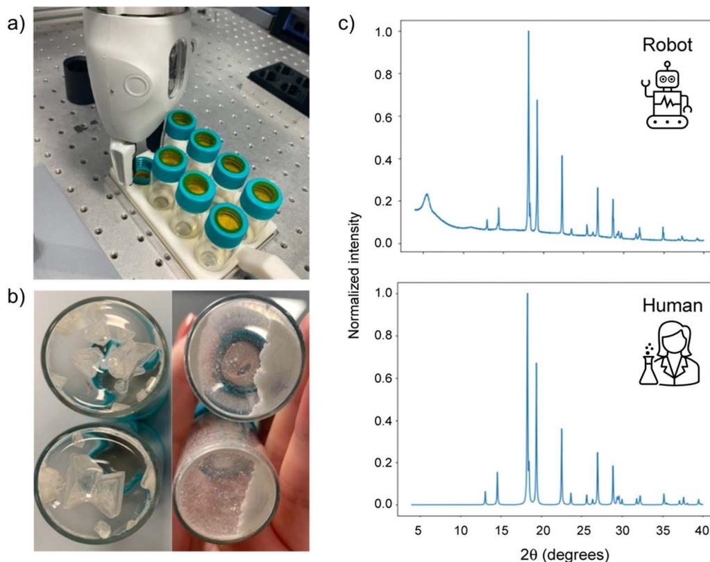
Fig. 8 Automated polymorph screening procedure. Crystals are grown in vials capped with Kapton tape to aid solid transfer (a). Samples are ground (b), then the vial caps are removed and analysed by PXRD (c). Adapted from ref. 140 with permission.
