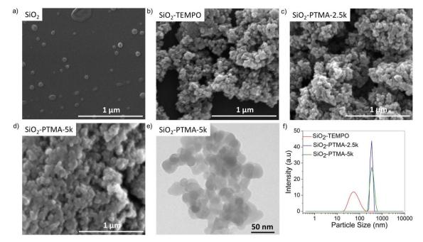
Fig. 2 FESEM micrographs of (a) SiO<sub>2</sub>, (b) SiO<sub>2</sub>-TEMPO, (c) SiO<sub>2</sub>-PTMA-2.5k, (d) SiO<sub>2</sub>-PTMA-5k, (e) TEM micrograms of SiO<sub>2</sub>-PTMA-5k, and (f) DLS of modified particles.
