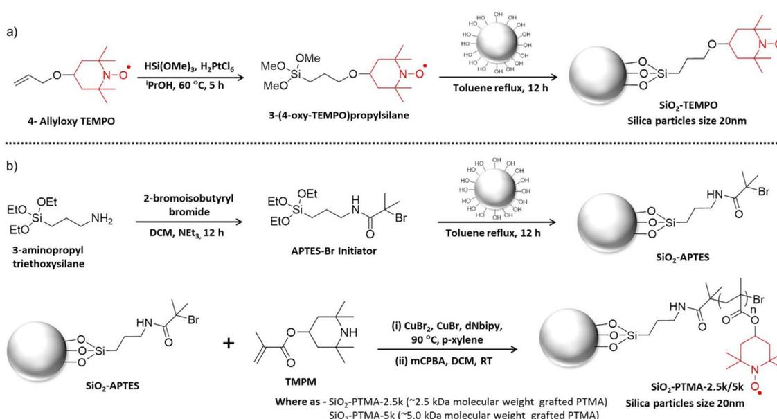
**Scheme 1** Modification of silica particles with (a) TEMPO units *via* direct functionalization; and (b) APTES-Br as initiator for SI-ATRP, subsequent grafting—from polymerization of PTMPM, and oxidation to access grafted PTMA.
