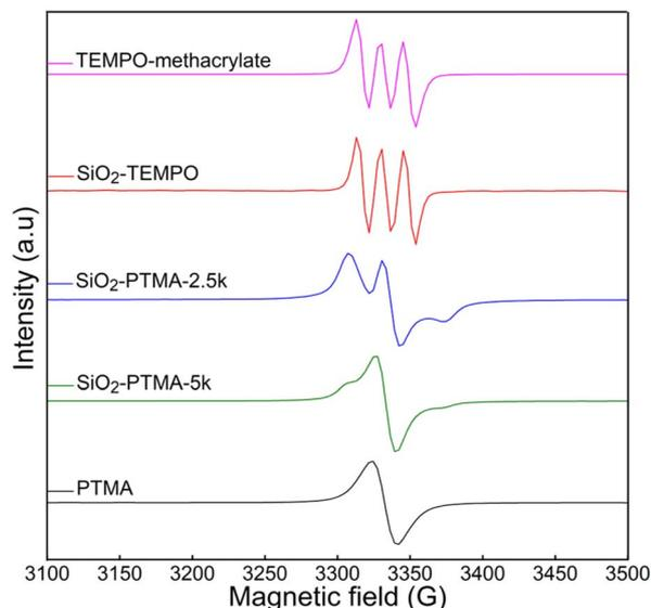
Fig. 3 EPR spectra of (from top to bottom) TEMPO methacrylate, SiO<sub>2</sub>-TEMPO, SiO<sub>2</sub>-PTMA-2.5k, SiO<sub>2</sub>-PTMA-5k, and PTMA.
