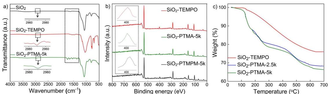
Fig. 1 Characterization of SiO<sub>2</sub>, SiO<sub>2</sub>-TEMPO, SiO<sub>2</sub>-PTMA-2.5k and SiO<sub>2</sub>-PTMA-5k by: (a) FTIR, (b) XPS, and (c) TGA.
