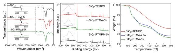
Fig. 1 Characterization of SiO<sub>2</sub>, SiO<sub>2</sub>-TEMPO, SiO<sub>2</sub>-PTMA-2.5k and SiO<sub>2</sub>-PTMA-5k by: (a) FTIR, (b) XPS, and (c) TGA
