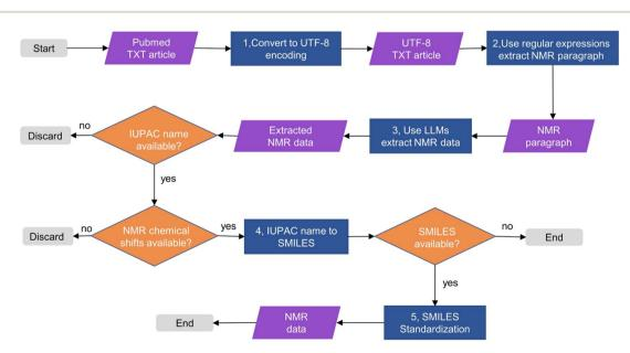
Fig. 2 The process of extracting NMR data from original research papers using NMRExtractor. Grey boxes represent starting and end points, purple parallelograms represent inputs and outputs, blue rectangles represent processing flows, and orange diamonds represent decision points in the pipeline.
