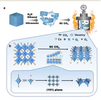
Fig. 1 (a) The process flow of SC CO $_2$  stripping on bulk phase CaTiO $_3$  (b) Schematic diagram of the effect of SC CO $_2$  on CaTiO $_3$ .
