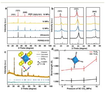
Fig. 3 Characterization of CaTiO $_3$  under different pressure treatments. (a) XRD. (b) Partially enlarged details of some planes. (c) The Rietveld-refined XRD patterns of CaTiO $_3$  under 16 MPa. (d) Variation in the bond length value of TiO $_6$  octahedra obtained by XRD refinement with increasing SC CO $_2$  pressure.
