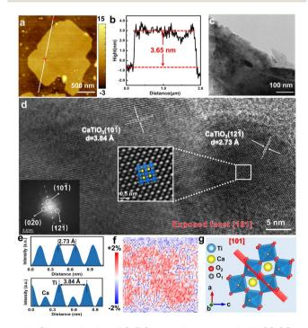
Fig. 2 Characterization of CaTiO $_3$  nanosheets treated with SC CO $_2$  at 16 MPa. (a) AFM image and (b) height profile of the line in (a). (c) TEM image. (d) HRTEM image. (e) The line contour of the plane spacing in (d). (f) The strain map demonstrate on the HRTEM image by geometric phase analysis (GPA). Strain-values from -2% to +2% can be represented when color changes from blue to red. (g) Atomic structure diagram of the (101) plane.
