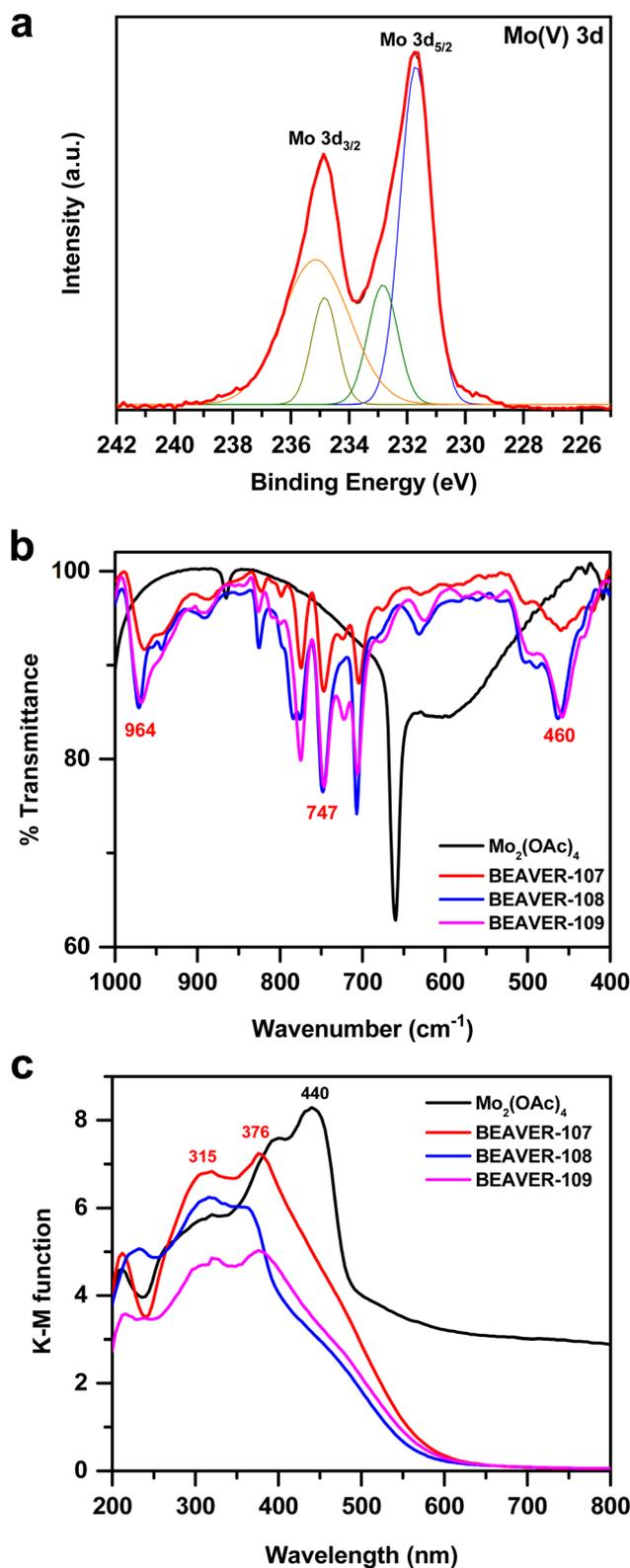
Fig. 2 Spectroscopic features of the Mo(v)-MOP molecule. (a) X-ray photoelectron spectra of BVR-107. (b) Fourier-transform infrared and (c) ultraviolet-visible spectra of Mo<sub>2</sub>(OAc)<sub>4</sub>, BVR-107, BVR-108, and BVR-109. All sets of spectra were recorded on the respective solids.
