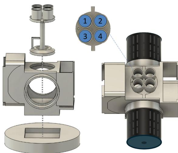
**Fig. 1** M-Arc reactor schematic (left). Hotplate base (bottom), photoreactor housing (middle), vial carousel (4 × microwave vial example) (top). LED lamp mounting of Kessil or HepatoChem EvoluChem lamps (right).
