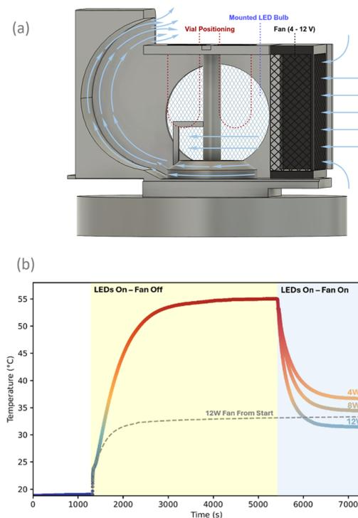
**Fig. 2** (a) Implementation of internal arc geometry to aid with airflow in the M-Arc reactor. (b) Temperature profile of M-Arc photoreactor when irradiated with 450 nm LEDs ( $2 \times 18$  W). A variable voltage fan confirmed the influence of fan power with reactor steady state temperature.
