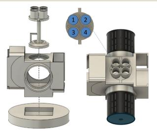
Fig. 1 M-Arc reactor schematic (left). Hotplate base (bottom), photoreactor housing (middle), vial carousel (4 × microwave vial example) (top). LED lamp mounting of Kessil or HepatoChem EvoluChem lamps (right).
