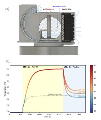
Fig. 2 (a) Implementation of internal arc geometry to aid with airflow in the M-Arc reactor. (b) Temperature profile of M-Arc photoreactor when irradiated with 450 nm LEDs (2 × 18 W). A variable voltage fan confirmed the influence of fan power with reactor steady state temperature.
