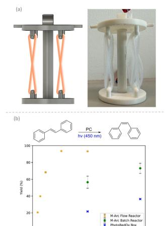
Fig. 5 (a) Figure-8 flow tubing fixation method (PTFE tubing, ID = 1.0 mm). (b) Kinetic uptake comparison of flow tubing in M-Arc reactor versus batch conditions in M-Arc and HepatoChem PhotoRedOx  $Rox^{TM}$
