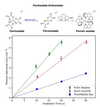
Fig. 3 Actinometric quantification of light delivery for M-Arc reactor and two commercial products (Asynt Illumin8 & HepatoChem PhotoRedOx Box<sup>TM</sup>).
