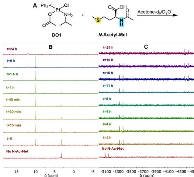
**Fig. 4** (A) Scheme of DO1 interaction with *N*-acetyl-met in deuterated solvent. (B) Time-dependent  $^{31}\text{P}$ -NMR (from  $t = 6$  to 20 h data not shown) of the sample A. (C) Time-dependent  $^{195}\text{Pt}$ -NMR of the sample (A).
