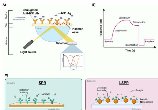
**Fig. 6** (A) Schematic representation of the general principle used in SPR biosensing, including a reflectance spectra at the detector. (B) Graphical representation of a generic SPR sensorgram, highlighting the steps involved in an analytical cycle.<sup>140,142</sup> (C) Schematic representation of differences between SPR and LSPR biosensing principles.<sup>147</sup> This figure was created in BioRender. Etienne, R. (2025) <https://BioRender.com/6k9p9i2>.
