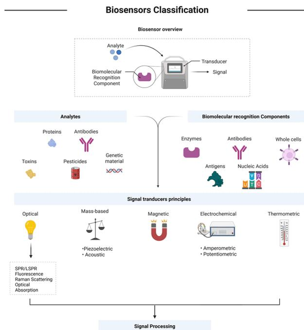
**Fig. 5** Graphical representation of the components included in an optical biosensor: a sensing unit, a signal transducing unit, followed by a processing unit, created in BioRender. Etienne, R. (2025) <https://BioRender.com/itw6yy0>. Adapted from Chen *et al.*<sup>76</sup>
