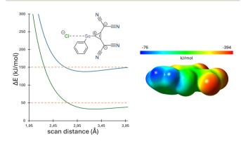
Fig. 3 Left: Total energy profile of the scan of the Cl-  $\cdot$  Se distance in the 8-Cl adduct in the gas phase (blue) and in MeCN solution (green) calculated at M06-2X level of theory. Right: Electrostatic potential of 8 mapped on the 0.001 electron/Bohr<sup>3</sup> isosurface of electronic density.
