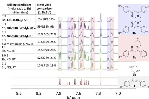
Fig. 3 Comparison of  $^1\text{H}$  NMR spectra (600 MHz,  $\text{CDCl}_3$ ) of (from bottom to top) starting materials, **1** and **2b**, with reaction mixtures collected after milling under different reaction conditions (molar ratios and milling time are depicted). Marks: two rectangles indicate the presence of two products; pink corresponds to single addition product **3b**, and blue to the double addition product **3b'**.
