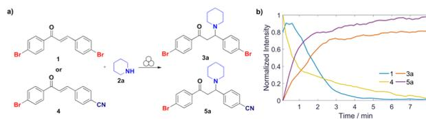
Fig. 2 (a) Impact of bromo and cyano substituents on the chalcone skeleton in aza-Michael addition of **2a** depicted with its corresponding (b) kinetics curves illustrating the formation of compounds **3a** and **5a**. The initially steady signal of **1** reflects slow homogenization of the reaction mixture at the onset of milling.
