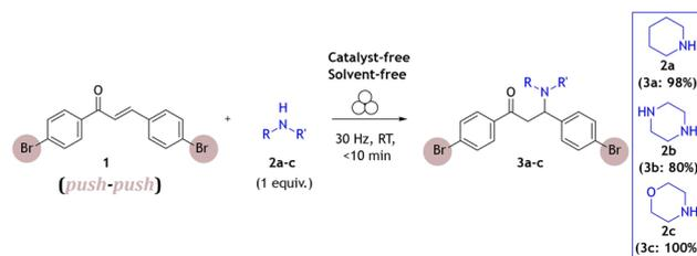
Scheme 1 Mechanochemical aza-Michael addition reaction of secondary cyclic amines **2a–c** to chalcone **1** performed in a vibratory ball mill. The yields were evaluated according to the <sup>1</sup>H NMR signals of reactants and the product.
