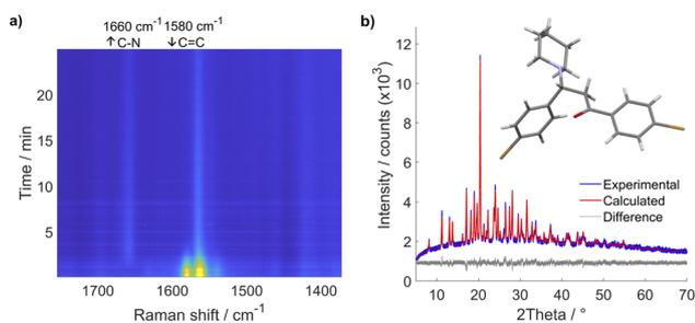
Fig. 1 (a) Time-resolved 2D Raman monitoring of milling **1** and **2a** in an equimolar ratio with two  $\text{ZrO}_2$  milling balls (mass 1.6 g, diameter 8 mm) in a vibratory ball mill at 30 Hz milling frequency. (b) Experimental diffractogram (blue line) of a powder collected immediately after milling and its Rietveld fit (red line) depicted with the solved crystal structure of **3a** (deposited under CCDC number: 2343064).
