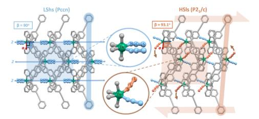
Fig. 3 Symmetry-breaking ferroelastic transition. Change of crystalline symmetry from the LT parent-paraelastic LShs Pccn phase to the HT daughterferroelastic HSIs P2<sub>1</sub>/c phase. The 2-fold molecular axes (2) along c in the LShs state are lost in the HSIs phase, which is associated with a shear of the molecular layers (orange arrows) opening the  $\beta$  angle, and an asymmetric torsion of the PM-PEA ligands and thiocyanate groups (NCS zoom).
