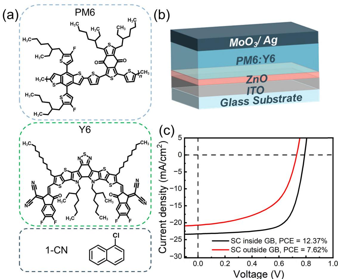
**Fig. 1** Materials, device architecture, and reference devices. (a) Molecular structures of components PM6, Y6, and 1-CN. (b) Sketch of the device stacking corresponding to the inverted structure. (c) Current density–voltage ( $J$ – $V$ ) curves of a representative SC PM6:Y6 OPV fabricated inside (black) and outside (red) the glovebox (GB), showing  $PCE_{avg}$  values.
