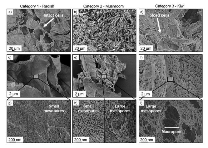
Fig. 4 SEM images of selected samples (radish, mushroom, and kiwi) from different sample categories obtained at different magnifications: (a)–(c)  $250\times$ ), (d)–(f)  $5000\times$ , (g)–(i)  $150000\times$ .
