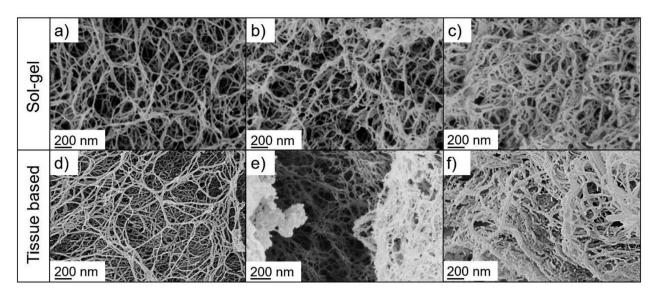
Fig. 5 Pore structures of calcium-ion crosslinked, pectin aerogels produced via the sol route (top, Reprinted from<sup>81</sup> with permission from Elsevier, Copyright 2018) and various tissue based samples produced in this work (bottom). Sol-gel based samples were produced with different pectin-contents in the sol: (a) 2 wt%, (b) 4 wt%, and (c) 6 wt%. Represented pore structures from tissue-based samples are: (d) nectarine (e) strawberry and (f)
