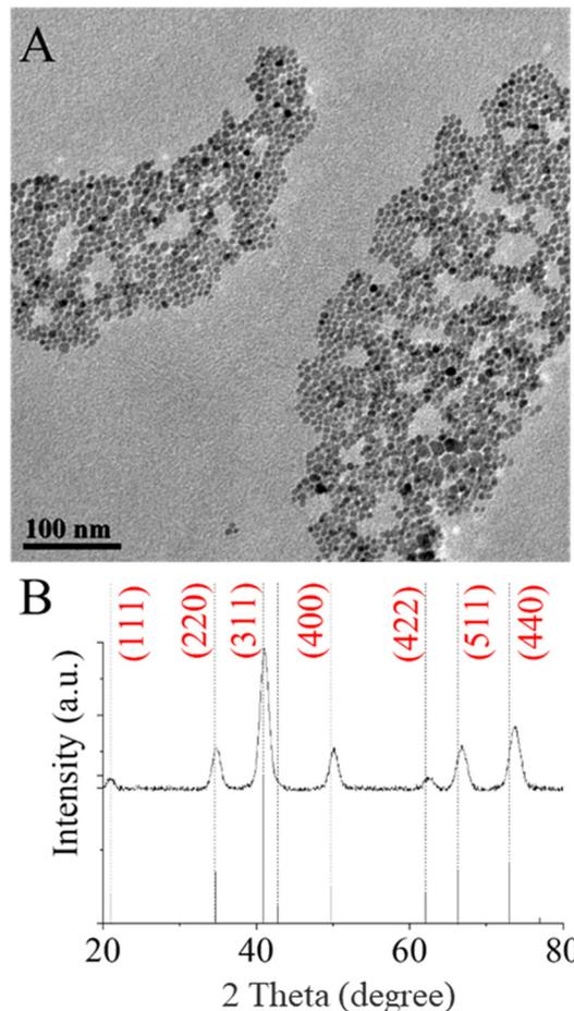
Fig. 1 Mn<sub>0.2</sub>Fe<sub>2.8</sub>O<sub>4</sub> NPs prepared at 250 °C for 6 h: (A) TEM images and (B) XRD patterns, and XRD reference for MnFe<sub>2</sub>O<sub>4</sub> (PDF card no 00-010-0319).
