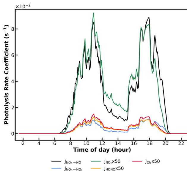
Fig. 1 Selected average photolysis rate coefficients (*J*) from measurements located both in the kitchen and living room, representing the outdoor attenuated light experienced inside the house:  $J_{\text{NO}_3 \rightarrow \text{NO}}$  (black line),  $J_{\text{NO}_3 \rightarrow \text{NO}_2}$  (blue line),  $J_{\text{NO}_2} \times 50$  (green line),  $J_{\text{HONO}} \times 50$  (yellow line), and  $J_{\text{Cl}_2} \times 50$  (red line).
