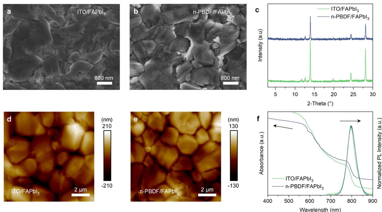
Fig. 2 SEM images of perovskite (FAPbI<sub>3</sub>) grown on (a) ITO and (b) n-PBDF electrodes on the glass substrate. (c) XRD spectra of perovskite grown on the ITO and n-PBDF electrodes. AFM height images of perovskite grown on the (d) ITO and (e) n-PBDF electrodes. (f) UV-vis and PL spectra of perovskite grown on ITO and n-PBDF electrodes.
