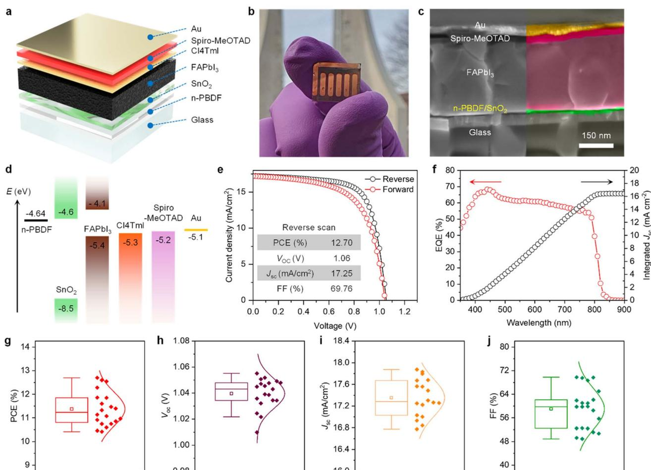
**Fig. 3** (a) Schematic and (b) photograph of the rigid n-PBDF-based PSC device. (c) Cross-sectional SEM image of the device with the structure of glass/n-PBDF/SnO<sub>2</sub>/perovskite (FAPbI<sub>3</sub>)/Cl4TmI/spiro-MeOTAD/Au. (d) Energy band alignment of the component layers in the n-PBDF-based PSC. (e)  $J$ - $V$  characteristics and (f) EQE with corresponding integrated  $J_{sc}$ . (g-j) Statistical results of the rigid n-PBDF-based PSC devices (from three batches,  $n = 20$ ).
