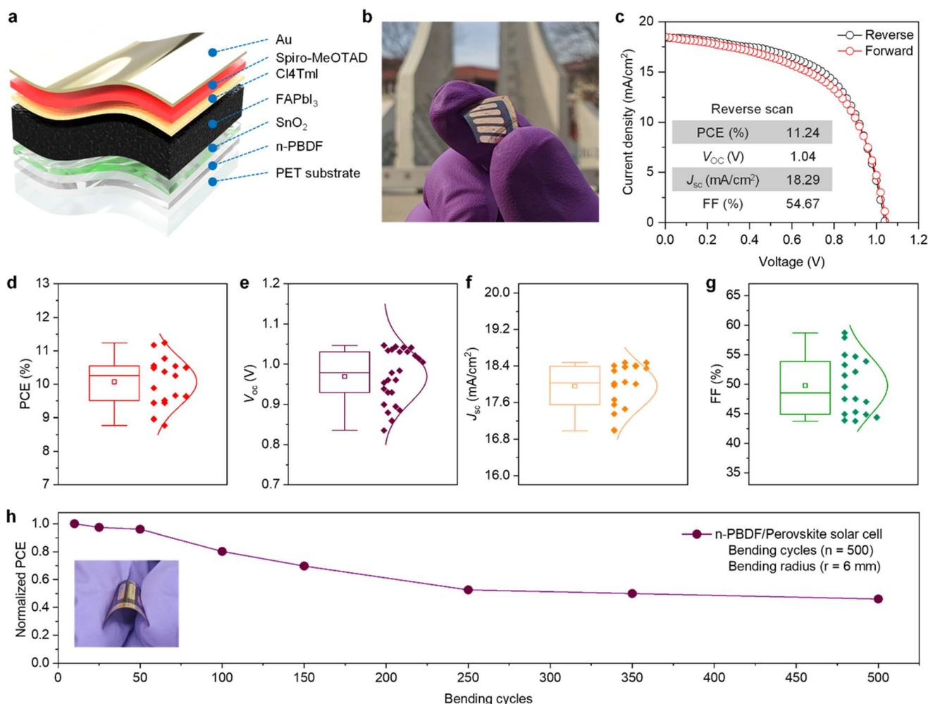
Fig. 4 (a) Schematic and (b) photograph of the flexible n-PBDF-based PSC device. (c)  $J$ - $V$  characteristics and (d–g) statistical results of the flexible n-PBDF-based PSC devices (from three batches,  $n > 18$ ). (h) Bending cycle stability test of the flexible n-PBDF-based PSC device.
