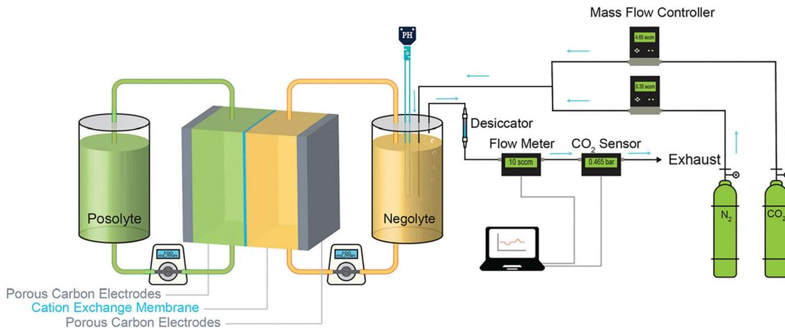
Fig. 7 Schematic of  $\text{Fe}(\text{CN})_6$  (posolyte)|DSPZ (negolyte) flow cell for  $\text{CO}_2$  capture/release experiments. Reproduced from ref. 141 with permission from the Royal Society of Chemistry, copyright 2020.
