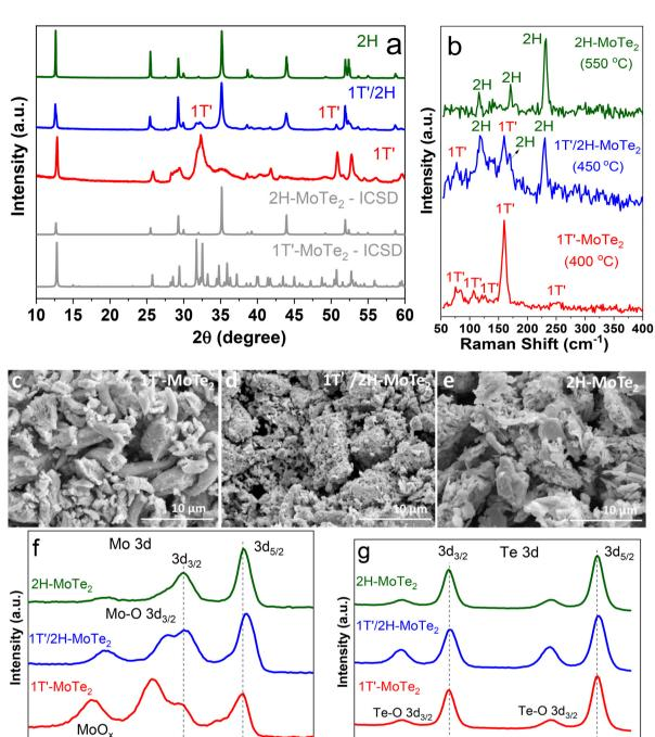
Fig. 1 (a) PXRD patterns of  $MoTe_2$  at different temperatures. (b) Raman spectra confirm the formation of  $1T'-MoTe_2$ , mixed  $1T'/2H-MoTe_2$  and  $2H-MoTe_2$  phases. SEM images of (c)  $1T'-MoTe_2$ , (d) mixed-phase  $1T'/2H-MoTe_2$  and (e)  $2H-MoTe_2$ . XPS spectra of  $MoTe_2$  showing (f) Mo 3d and (g) Te 3d peaks at different annealing temperatures.
