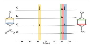
Fig. 3 <sup>1</sup>H NMR spectra of: (a) commercial 4-nitrophenol (5.0 mM) and commercial 4-aminophenol (5.0 mM) in the presence of NaBH<sub>4</sub>, before catalyst addition (1.3 M); (b) commercial 4-aminophenol (5.0 mM) in the presence of NaBH<sub>4</sub> (1.3 M); (c) commercial 4-nitrophenol (5.0 mM) in the presence of NaBH<sub>4</sub> (1.3 M) before catalyst addition; and (d) after 15 minutes of reduction using mixed-phase 1T'/2H-MoTe<sub>2</sub> catalyst (14 mM).
