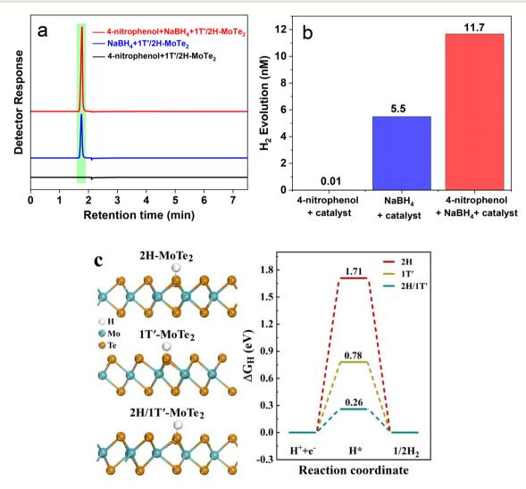
Fig. 4 (a) Headspace gas chromatography measurements and (b) hydrogen evolution after 15 minutes of reaction for 4-nitrophenol + 1T'/ 2H-MoTe<sub>2</sub> catalyst, NaBH<sub>4</sub> + 1T'/2H-MoTe<sub>2</sub> and 4-nitrophenol + NaBH<sub>4</sub> + 1T'/2H-MoTe<sub>2</sub> catalyst. (c) The optimized structural configuration of H adsorbed on MoTe<sub>2</sub> monolayers with 2H, 1T', and 2H/1T' phases and the associated free energy diagram.
