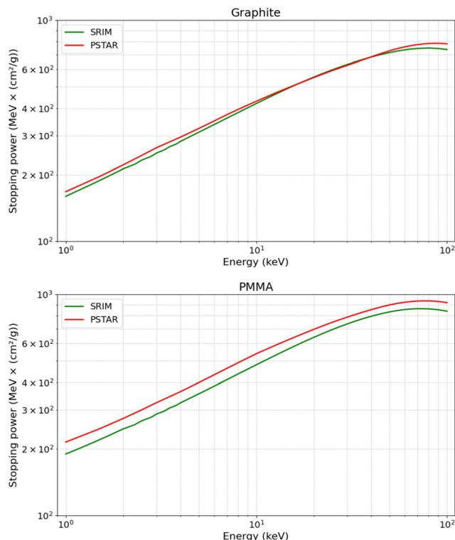
**Fig. 5** Comparison of the stopping power of protons in graphite and PMMA over the kinetic energy range of 1 keV to 100 keV.
