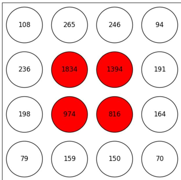
Fig. 7 MD simulation results showing the maximum kinetic energy of the PKA in the highlighted area of Fig. 6, expressed in kcal mol<sup>-1</sup>.
