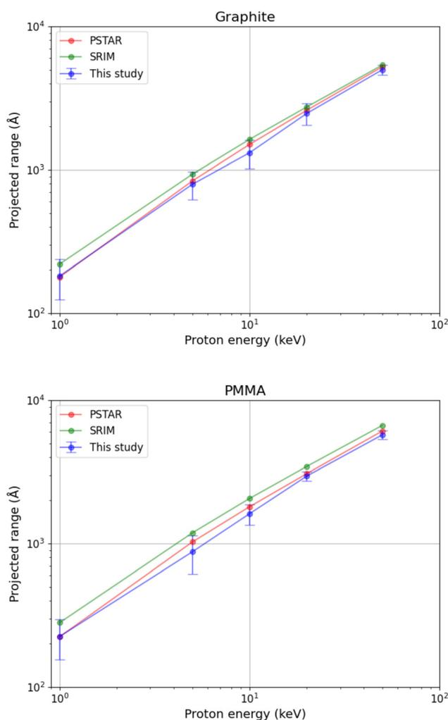
**Fig. 4** Comparison of the projected range of protons in graphite and PMMA calculated in this study with reference data from PSTAR and SRIM. Error bars represent one standard deviation.
