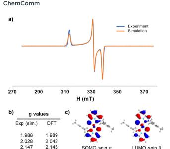
Fig. 4 (a) X-band EPR spectrum of the electrochemically generated [3]+ in frozen CH<sub>2</sub>Cl<sub>2</sub>/toluene solution (+0.1 M TBAP) at 110 K. Microwave frequency = 9.417556 GHz, mod. ampl. = 0.2 mT, and power = 6.4 mW. (b) q values obtained by simulations<sup>15</sup> and DFT calculations. (c) DFToptimized structure of  $[\mathbf{3}]^+$  and representation of the SOMO spin  $\alpha$  and LUMO spin  $\beta$  (isodensity value of 0.05 a.u.).
