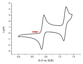
Fig. 3 Anodic cyclic voltammogram of complex 3 (Glassy carbon working electrode, 1 mM in CH<sub>2</sub>Cl<sub>2</sub> with 0.1 M Bu<sub>4</sub>NPF<sub>6</sub> as the supporting electrolyte, 100 mV s<sup>-1</sup> scan rate; potentials were calibrated against Fc<sup>+</sup>/Fc used as an internal standard with  $E_{1/2}$  (Fc<sup>+</sup>/Fc) = 0.46 V vs. SCE)
