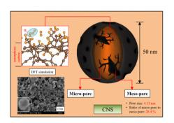
Glucose-based highly-porous activated carbon nanospheres (g-ACNSs) for high capacity hydrogen storage
