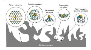
Understanding the role of nitrogen-doping and surface topology in the binding of Fe(III)/Fe(II) to biobased carbon electrodes
