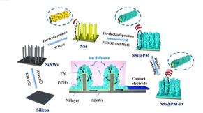
Passivation of silicon nanowires with Ni particles and a PEDOT/MnO<sub>X</sub> composite for high-performance aqueous supercapacitors
