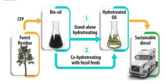
Diesel production via standalone and co-hydrotreating of catalytic fast pyrolysis oil
