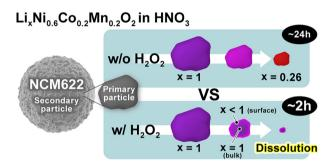
Mechanisms underlying the acid leaching process for LiNi<sub>0.6</sub>Co<sub>0.2</sub>Mn<sub>0.2</sub>O<sub>2</sub> with and without H<sub>2</sub>O<sub>2</sub>
