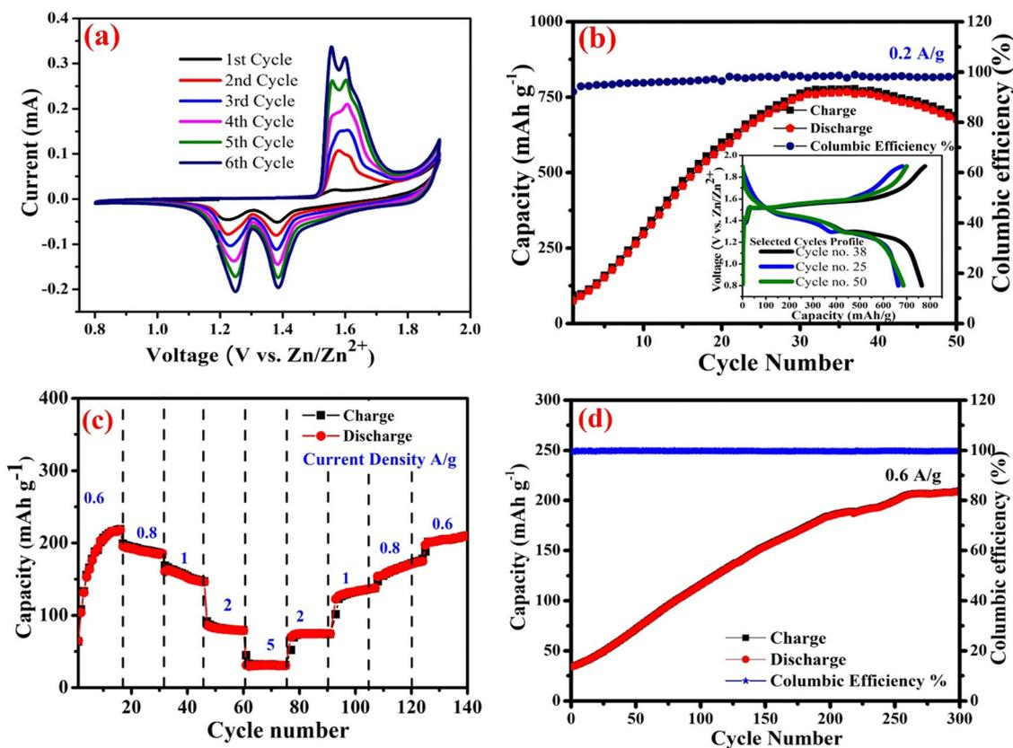
Fig. 3 Electrochemical performances of the  $\text{Mn}_3\text{O}_4$  nanoparticles cathode: (a) CV curves at a scan rate of  $0.1 \text{ mV s}^{-1}$ , (b) cycle performance at  $0.2 \text{ A g}^{-1}$  and inset is discharge/charge profiles of selected cycles, (c) rate property, and (d) cycling performance at  $0.6 \text{ A g}^{-1}$ .
